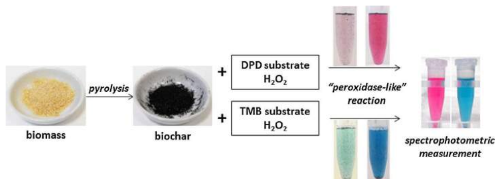
Fig. 1 Scheme of biochar preparation and its peroxidase-like activity determination using DPD and TMB co-substrates in the presence of hydrogen peroxide, followed by spectrophotometric measurement of the colored reaction product (color online)
